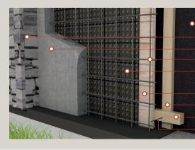
the battens. Drainage of any moisture must be inserted in the air gap between the wind barrier and OSB panel. This consists of a 22 mm draft pipe (electrical pipe) which is laid out hidden between the slate at the bottom of the dry wall and bent up behind the cross batten.
