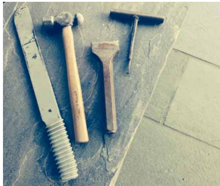
TOOLS FOR SHAPING CRAZY PAVING TILES
